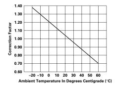
To use this chart: Read up from the ambient temperature to the curve, and across to find a correction factor. Multiply the breaker rating by the correction factor to determine the compensated rating. Calculate the overloads in terms of the compensated rating to use the published trip curve. Do not use these devices outside their specified operating temperature ranges.
